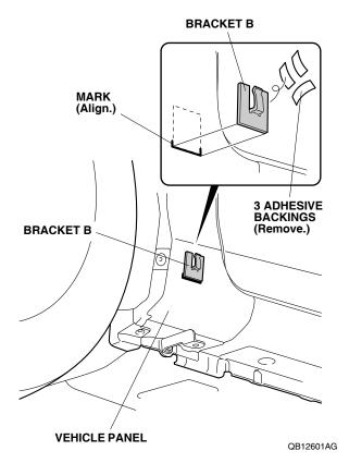
12. Align bracket B with the mark made in step 10, and attach it to the vehicle panel. Press and hold the bracket firmly against the vehicle for 30 seconds.
