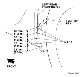
6. Using a utility knife, remove any sealant on the inside of the left rear fenderwell in the area shown. Be careful not to damage the paint finish.
