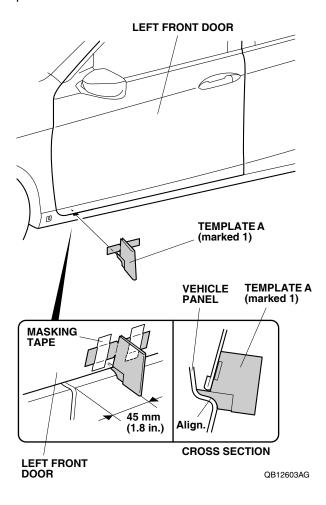
16. Using a felt-tip pen, mark the vehicle panel at the measurement shown.
