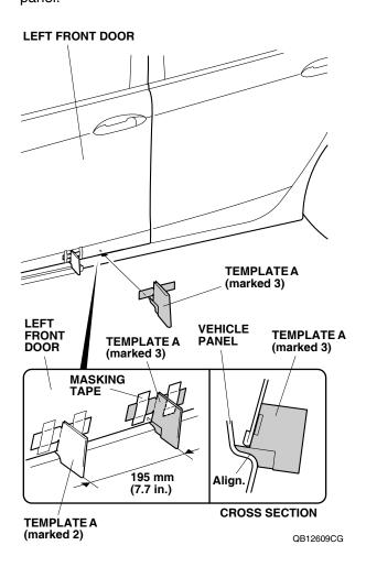
23. Using a felt-tip pen, mark the vehicle panel at the measurement shown.
