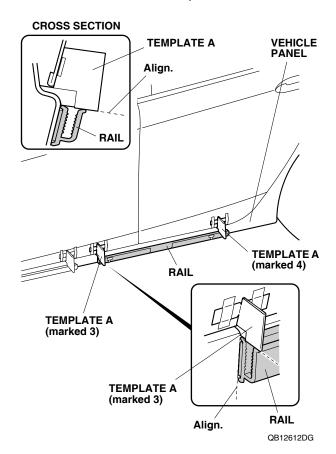
28. Make sure that the rail is aligned with each template, then carefully remove each adhesive backing.
