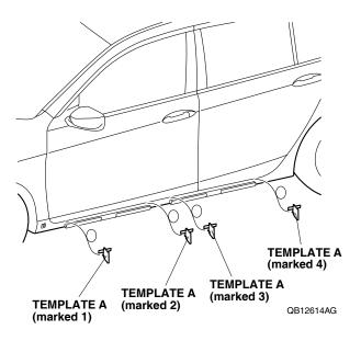
30. Using the palm of your hand, firmly press the rails against the vehicle panel for 30 seconds. Remove the marks you made using isopropyl alcohol on a shop towel.
