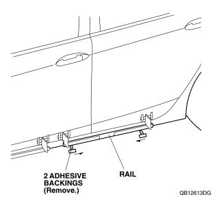
29. Remove all four templates. Be careful not to damage the templates. They are also used to mark the right side of the vehicle.
