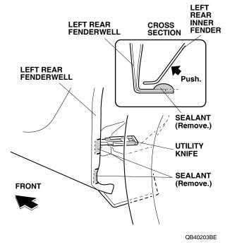
7. Apply touch-up paint to the areas where you removed the sealant, and allow it to dry thoroughly.
