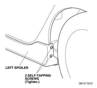
48. Tighten the bracket screw.
