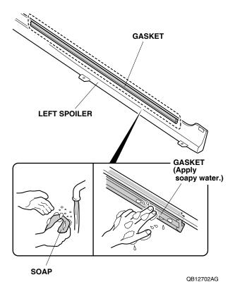
33. Secure the hook on the left spoiler to bracket B and align the gasket on the left spoiler with the rails. Insert the front end of the gasket into the rail first, then work rearward. Move the left spoiler up and down gently to make sure that the gasket is installed securely to the rails.
