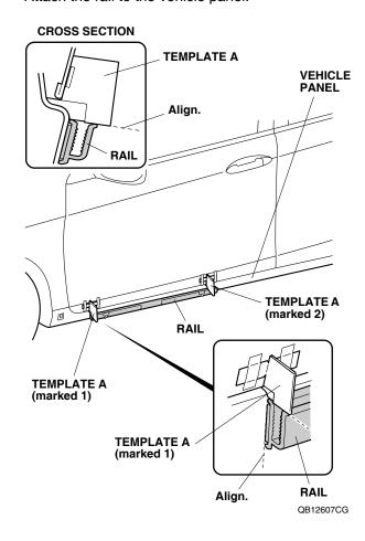
21. Make sure that the rail is aligned with each template, then carefully remove each adhesive backing.
