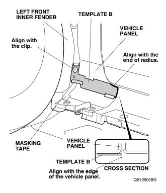
10. Using a felt-tip pen, mark the vehicle panel in the area shown. Remove template B. Be careful not to damage the template. It is also used to mark the right side of the vehicle.
