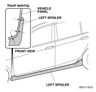
35. Lightly tap the left spoiler to remove any gap between the left spoiler and the left rear fenderwell.
