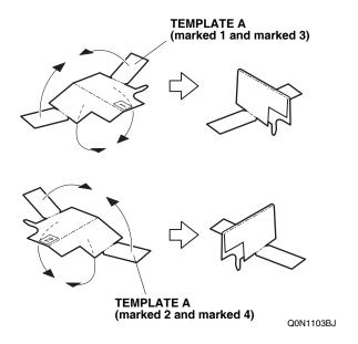
15. Place template A (marked 1) into position at the location shown. Align template A with the vehicle panel; lightly push down on the template, and attach it to the left front door with masking tape. Make sure there is no gap between the template and the vehicle panel.
